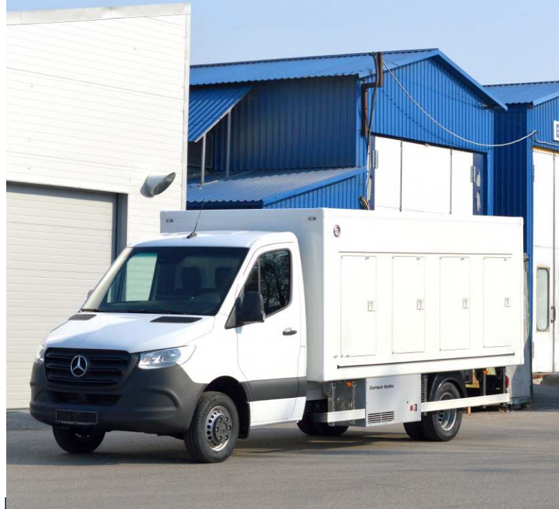
Body with increased volume vs. standard 12-door body
